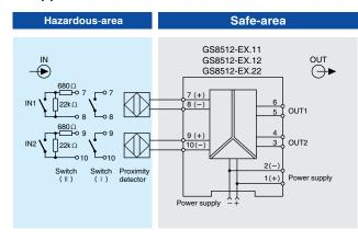
Note: GS8512-EX.11,only contains input1, output1; GS8512-EX.12 the input part only contains input 1.
